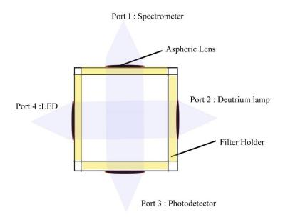
All ports are Interchangable & have option to use SMA fiber & directly atttach using optics to minimize insertion loss & other losses
