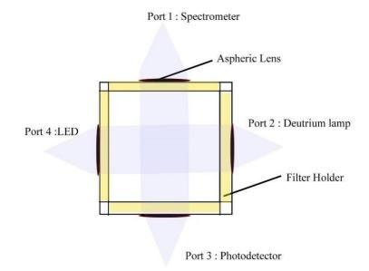
All ports are Interchangable & have option to use SMA fiber & directly atttach using optics to minimize insertion loss & other losses
