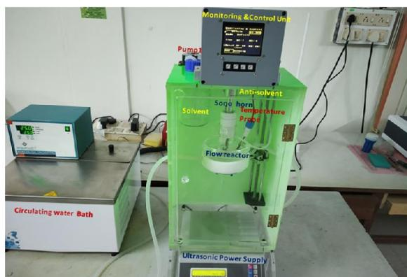
Working prototype of semi automatic temperature and flow control ultrasonic spray system consists of (i) Ultrasonic power supply with sonohorn probe (ii) Double wall glass reactor with inlet and outlet (iii) Temperature Probe (iv) Microcontroller based monitoring and control module (v) Peristaltic Pump 1 & 2 (vi) Reagent Bottle 1 (solvent) & 2 (anti-solvent) (vii) mechanical assembly for support and adjust the position of reactor (viii) Circulating water bath
