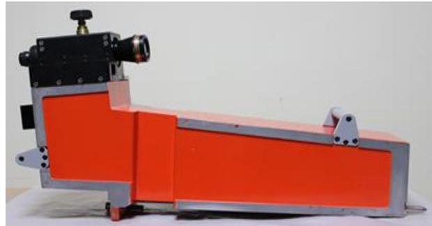
used to install and harmonize cockpit display and optronic systems at the desired position in the aircraft cockpit with reference to the aircraft axis (Fuselage Reference Line - FRL). It provides harmonization capability within tolerance of 1mR for harmonization distance of 60m. With this accurate harmonization, the target positioning for these Optronic Equipment would be within 9 feet for a distance of 20 kms.
