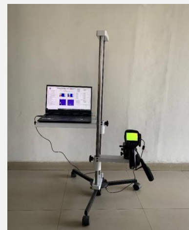
Thermal imaging based non-invasive system for diagnosis of Knee OA
