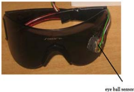
Figure 2: The Eyeball Sensor on goggles
