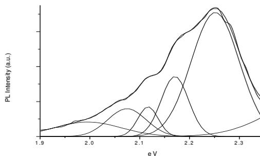
Figure 3: Smoothed and curve fitted PL spectrum of copper oxide NPs
