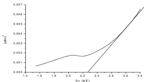
Figure 4: Tauc plot for as synthesized NPs solution of NPs. The best linear relationship is obtained by plotting  $(\alpha h\nu)^2$  against  $h\nu$  indicating that the optical band gap of these colloidal NPs is due to a direct allowed transition. The value of the band gap is determined from the intercept of the straight line at  $\alpha$
