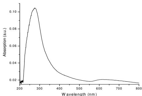
Figure 2: UV-VIS absorption spectrum of as synthesized colloidal NPs
