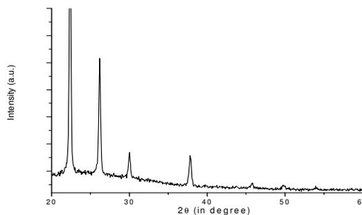
Figure 1: XRD spectrum of as synthesized NPs
